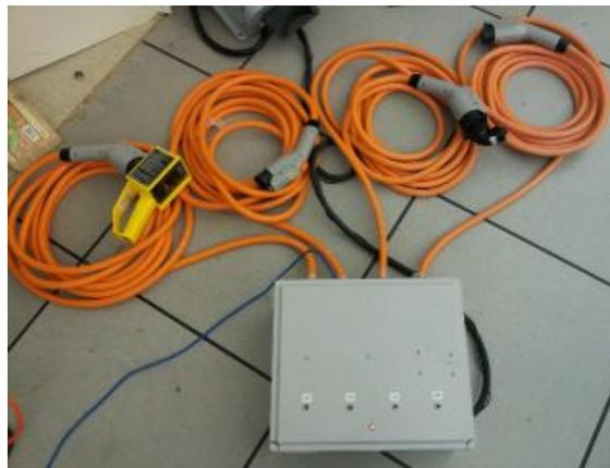
Fig. 4: Realization of 4 channel charging station
