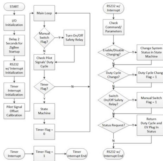
Fig. 8 Pilot signal monitor firmware flow chart
