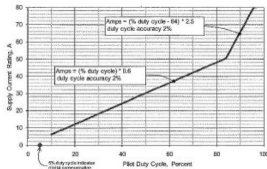
Fig. 5: Supply current v.s. pilot duty cycle[12]
