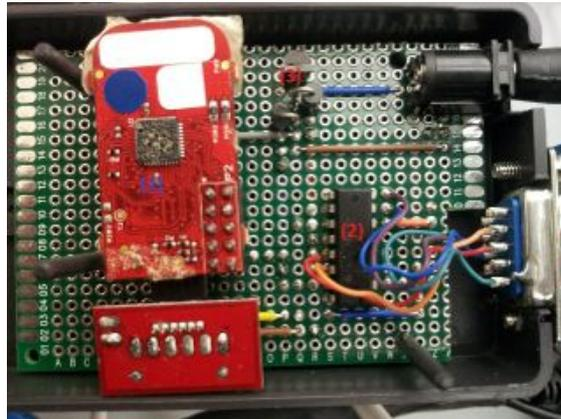
Fig. 12: ZigBee coordinator implementation: (1) ZigBee CC2530ZNP (2) MAX3232
