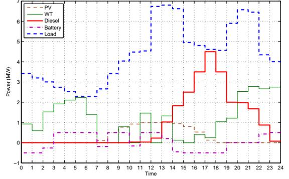
Fig. 6. Output schedules in grid-connected mode.
