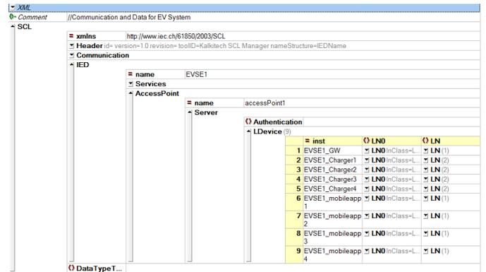
Fig. 2 Communication & Data Modeling using IEC61850
