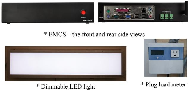
Fig. 3. ESI testbed - pictures of the EMCS and two types of energy loads.
